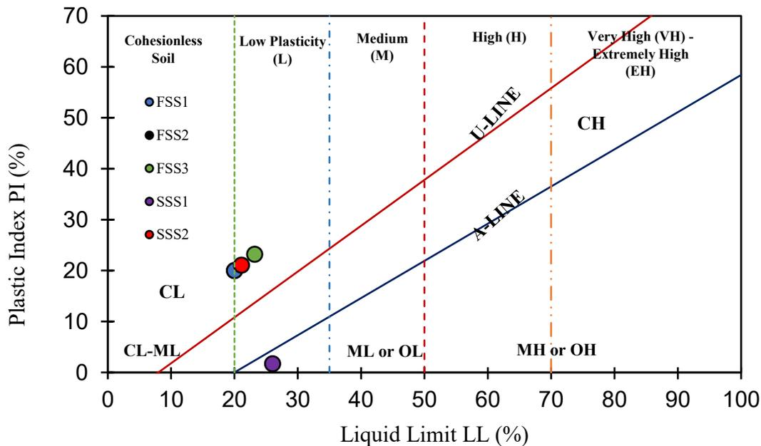
Figure 4: Plasticity Chart for the Tested Soil Samples
