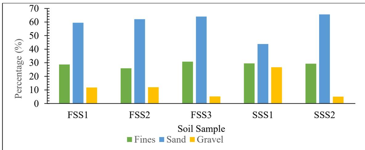
Figure 3: Percentage of Soil Types across the Stable and Failed Soil Samples
