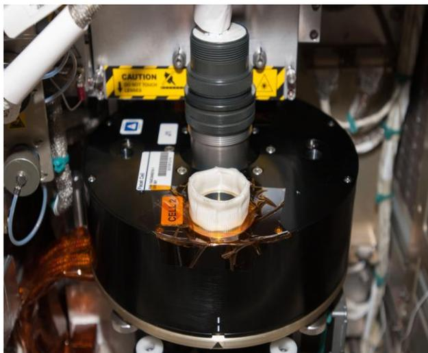
Figure 1: NASA Image: ISS040E019216 - Photographic documentation of the installation of the Soret-Facet into the Solution Crystallization Observation Facility (SCOF) inside the Ryutai rack in the Japanese Experiment Module (JEM) aboard the International Space Station (ISS)
