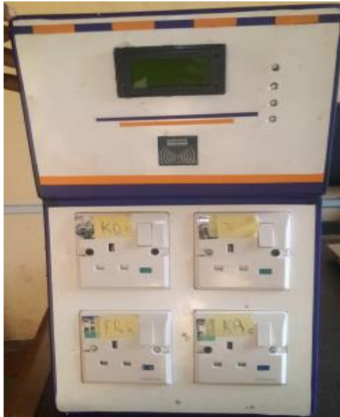
Figure 9: The Multi-user Prepaid Meter Complete Project with Casing
